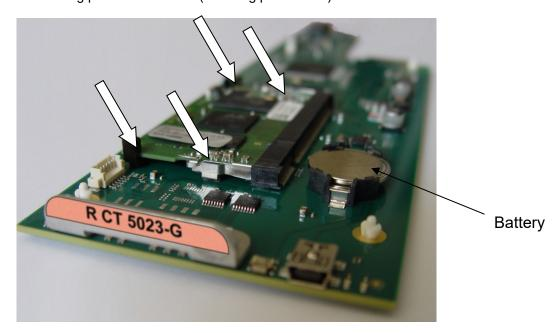
3. Insert the battery into the battery holder on the R CT 5023 module
