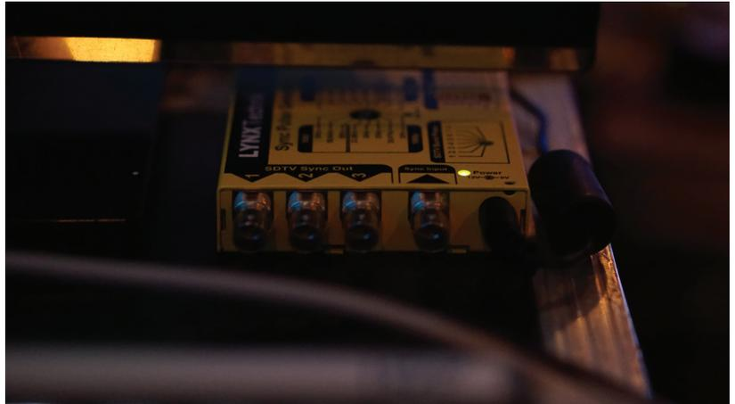
The whole SDI broadcast setup was synchronized to the master clock generated by the yellobrik HD / SD Sync Pulse Generators with Genlock.
