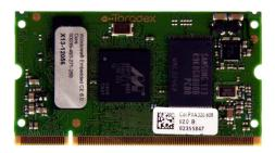
The OH\_RCT5023\_SERVER option is an independent Linux Server with its own IP-address. For power and LAN connection it is clipped as a piggyback onto the R CT 5023 controller card.
