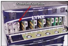
The rack frame terminal connector has a total of five RJ45 connectors. Depending on the type of controller that is inserted into the frame, these connectors are active or not. However, now with the new R CT 5023 controller card design, the top four connectors that are highlighted green (Control I/O) and blue (Extend I/O) are only required for legacy controller cards (for details regarding legacy controllers please read the Control System Overview Rev 1).
