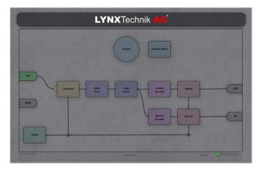
The main page of the Web UI reflects the functional diagram of the module. To access the detailed settings, double click on the respective functional block in the diagram and the configuration page will open. Use the back button to return to the main page.
