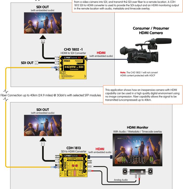
Note: CDH 1813 overlay mode can be switched on or off. Overlay is monitoring only, the module does not generate timecode or metadata.
