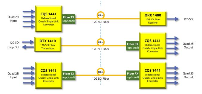
A fiber Transceiver option is also available. This includes both a Transmitter and Receiver in a single SFP package. The receive and transmit functions cannot be used simultaneously, but this option is useful if the CQS 1441 configuration is frequently changed where fiber transmission is sometimes needed and on other occasions fiber reception.
