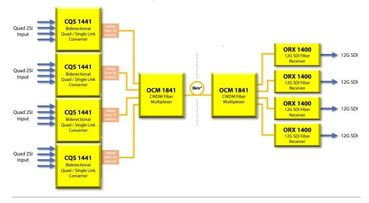
This application shows 2x CQS 1441 being used bidirectionally over a single fiber link as well as combining ethernet or serial RS232/422into the same link.
