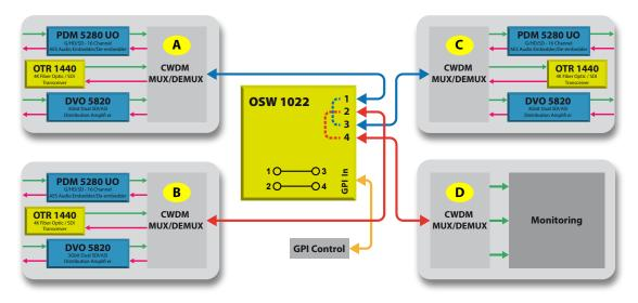
State 2: In this connection path, MUX A is connected to MUX D and MUX B is connected to MUX C.
