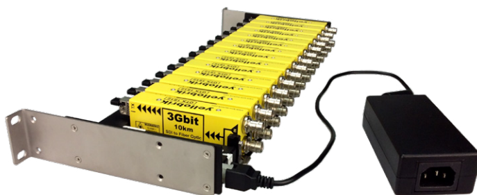
Rear of rack frame showing power connectors and one optional external power brick (use second brick for redundant protection)
