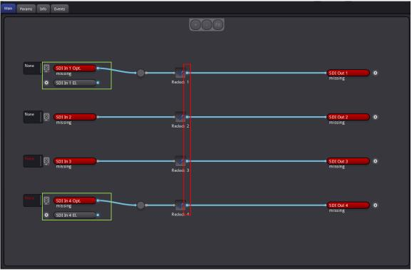
The input detection indicates the bit rate (SD-SDI = 270MBit/s, HD-SDI = 1.5 GBit/s; 3G-SDI = 3GBit/s) of a connected signal. If no signal is detected the color of the input detection will turn red and indicate a missing signal.
