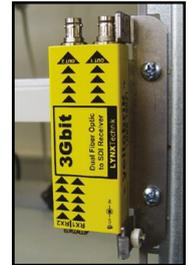
The optional RFR 1000-1 rack mount can be used to permanently mount up to 14 yellobrik modules. In addition, the RFR 1000-1 can provide full power redundancy for all mounted yellobrik.
