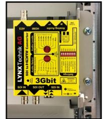
The optional RFR 1000-1 rack mount can be used to mount up to 14 yellobriks. In addition, the RFR 1000-1 can provide full power redundancy for all mounted yellobriks.
