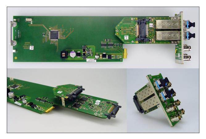
Those of you familiar with fiber interface cards will note the absence of the familiar "service loop" of fiber cable coiled around on top of the card. Using SFP sub modules removes the need for a service loop and improves serviceability. The SFP sub modules can be easily exchanged or upgraded for CWDM multiplexing applications.
