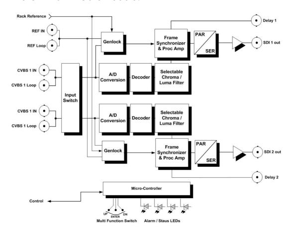
Figure 1- C AD 5112 Functional Diagram
