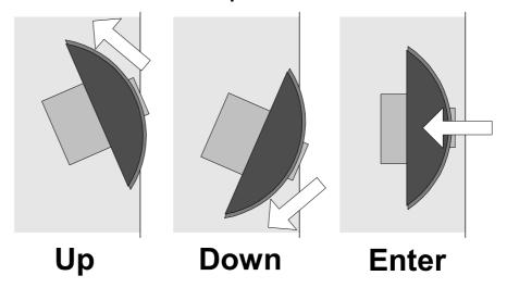
Figure 4 – Switch Operation
