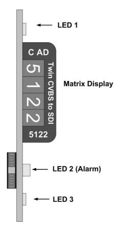
Figure 3 – Switch and Display Location
