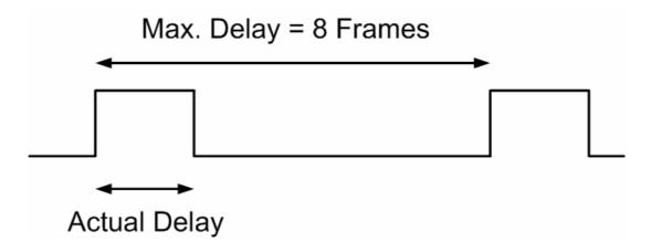
Min. Delay in Frame Synch Mode is 1 Frame Min. Delay in Line Synch Mode is < 1µs
