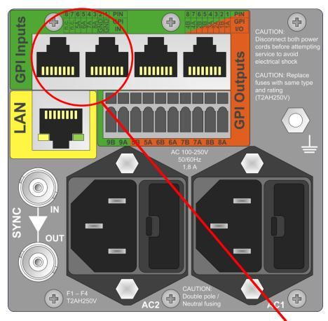
The two RJ45 connectors are looped through, so connections can be done through the one or the other connector Pinning of the RJ45 connectors is according to TIA/EIA 568-B.
