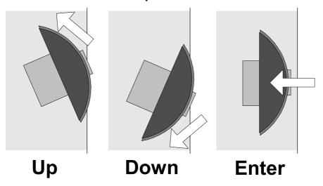
Figure 4 – Switch Operation
