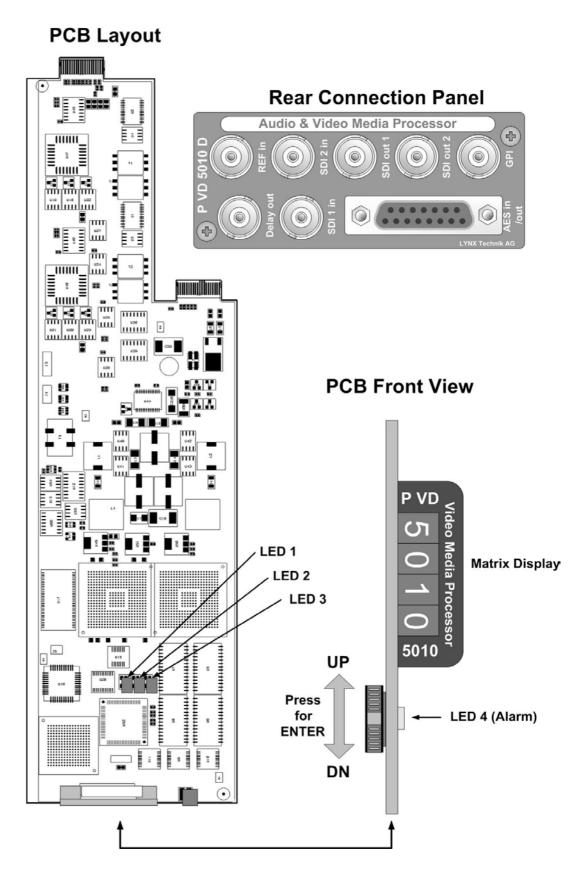
Figure 2: Physical layout P VD 5010 D
