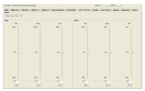
Gain amplifies the signal until it is clipped. Offset lifts the black level of the complete signal without impact on the gain.
