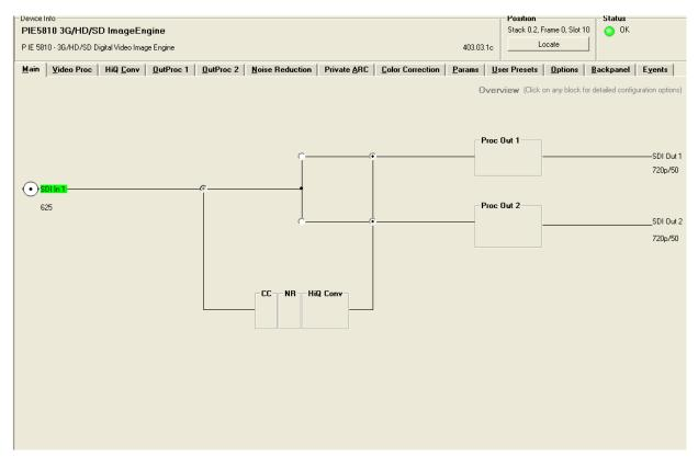
The primary purpose of this screen is to show the overall signal flow through the module and allow easy navigation to other areas. Input standards and formats are auto detected and displayed in the GUI. Parameters will be annunciated in different colors to show status (green = good, red = problem, yellow = caution etc).
