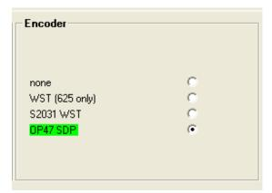
If WST teletext data is present / selected then the line numbers containing teletext data on both the input and output are shown. The green designation indicates valid teletext data is present.
