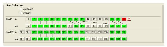
The encoder always tries to map the same input line to output line, in our example above line 17 and 19 are not used on the output as they were not used in the input. Clicking on these line numbers would activate their use in the output.
