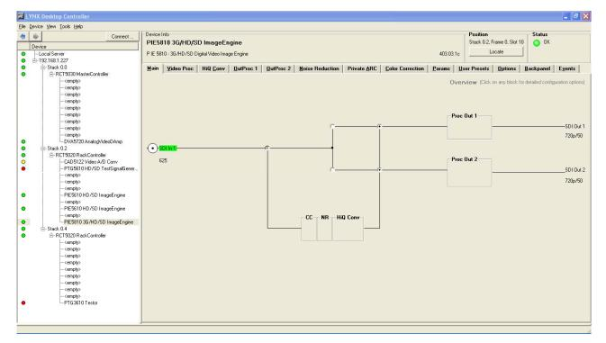
The above screenshot shows the complete module GUI. The Device info area contains information about the module including name and firmware revision. If used as part of a larger system (using the LYNX central control system) the modules position and physical location is displayed above the "locate" button.
