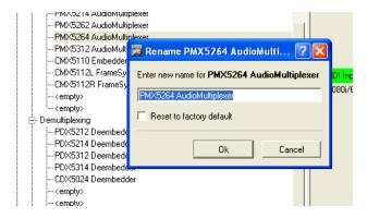
Simply type in the name you wish to assign to this device and press OK. If you wish to restore the default name simply select "Reset to Factory Default" and press OK
