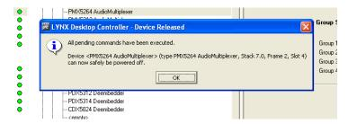
It is recommended you use the release function before removing any module from the rack to ensure the latest settings have been stored prior to module removal (if a module is removed before the normal 10 second timeout then the settings will not be stored)
