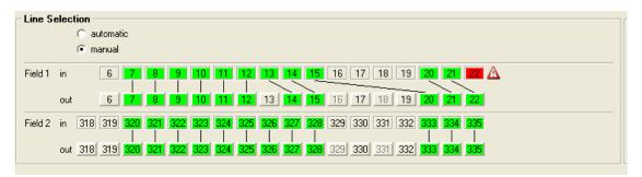
The encoder always tries to map the same input line to output line, in our example above line 17 and 19 are not used on the output as they were not used in the input. Clicking on these line numbers would activate their use in the output.
