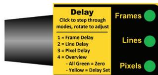
When an LED is illuminated turning the rotary control will adjust the delay in the selected increments (frames / lines / pixels).
