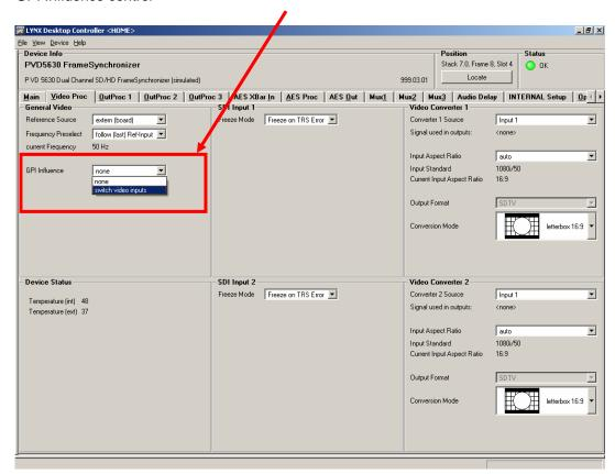
With GPI control enabled, the internal video cross bars are greyed out in the GUI and cannot be changed manually any longer, as the GPI control will steer the internal router to route the second input into the three available outputs so the output format configurations remain fixed – the only functional change is that the outputs are now being fed from the second input not the first. While not user accessible, the current status of the internal router can still be observed. See below.
