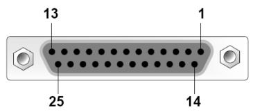
View looking INTO connector as seen on module
