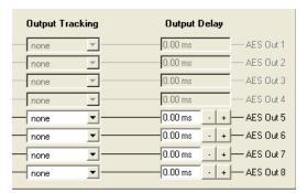
Use the drop down list provided to link the four external AES outputs to one SDI output channel auto tracking delay value.
