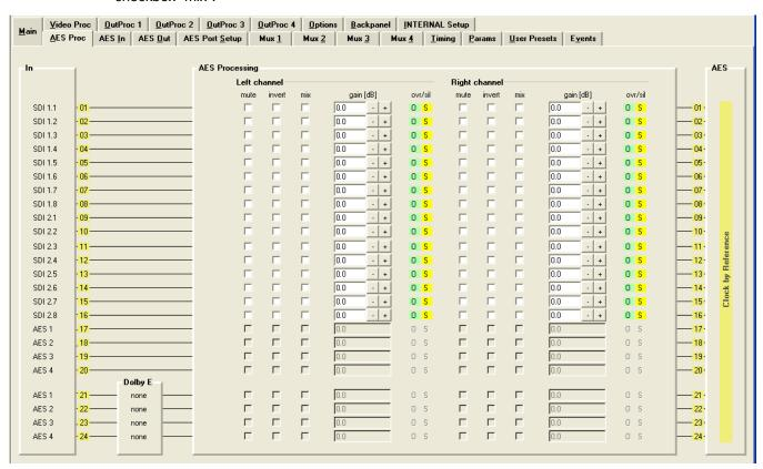
**Note:** If any Dolby E signal or other Audio data is passed through the processing stage, the processing will be deactivated, so the audio data will not be modified (controls will be greyed out). Settings will be set back to the original value if PCM audio will be switched to the same path.
