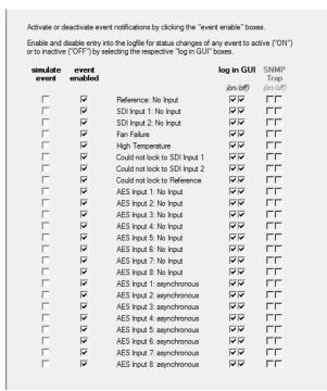
The GUI has an integrated error log, which is a simple text log file stored in the controller PC. This will record an event and timestamp it. The log can be seen at the bottom of the GUI screen and can be scrolled through using the scrolling bar.
