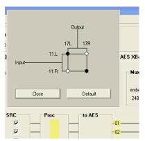
The Mini cross bar looks like shown, and permits full control over the routing of the left and right audio channels within the AES cross point selected.
