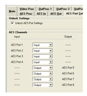
Note. The P VD 5822 is shipped with AES1..4 as inputs and AES 5..8 as outputs
