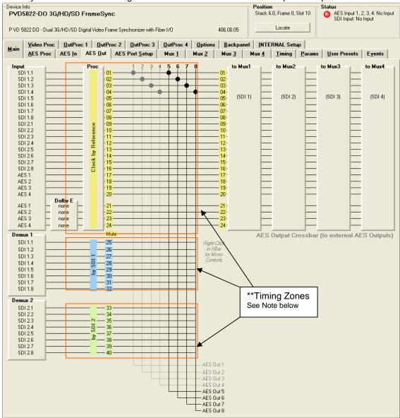
All inputs to the crossbar are shown horizontally and the 8 x External AES outputs are shown at the bottom of the screen. Selecting a cross point will route the required signal to the selected AES output.
