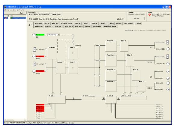
The above screenshot shows the complete module GUI. The Device info area contains information about the module including name and firmware revision. If used as part of a larger system (using the LYNX central control system) the modules position and physical location is displayed above the "locate" button.
