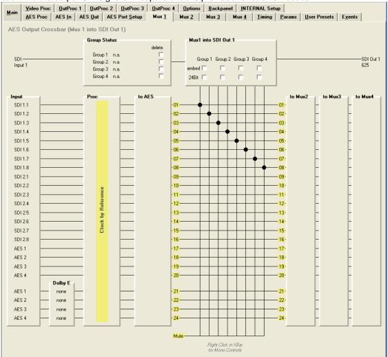
All of the internal audio from pathways 1 and 2 are made available as inputs to each embedder. The embedder can be seen at the top of the GUI and it's possible to quickly disable or enable an individual AES "Group" using the checkbox provided.
