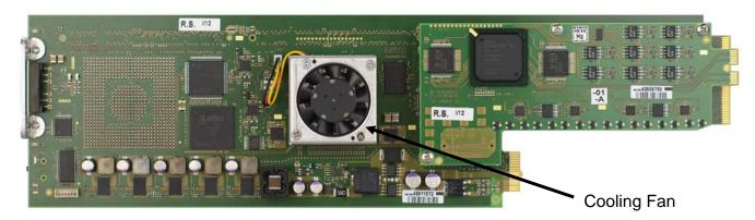
**Note.** Cooling fan operation is monitored and alarmed with the module alarm LED and also within the LYNX control system.
