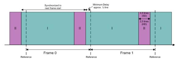
For distortion free switching in front of the P VD 5822, e.g. in a router, all signals have to be in area "I" or all signals in area "II".
