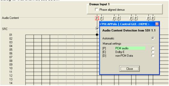
The default setting is always automatic, as seen above and for this first input you can see it has detected PCM audio.
