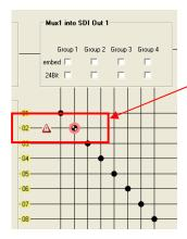
Here you can see the highlighted cross-point has been manually changed from its default settings. The warning symbol clearly indicates there is a conflict with this crosspoint setting for the audio signal present.
